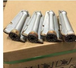
It is important when replacing a propane furnace to offer a stainless-steel burner option to customers up front. For one, they will offer reliability beyond stock burners, which in turn means fewer breakdowns. Second, burners are not covered under standard warranty, as they are considered maintenance items that should be cleaned routinely during a heat tune-up.
